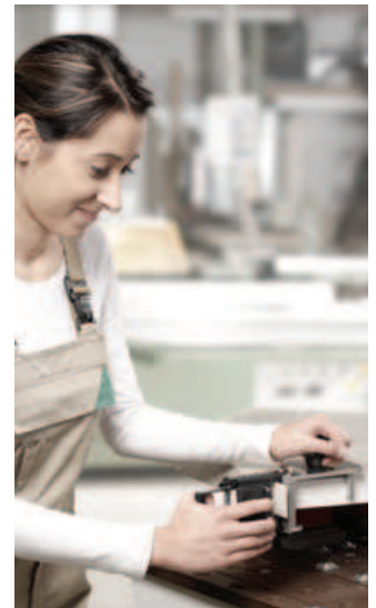
Placing the guillotine on the glued edgeband.
