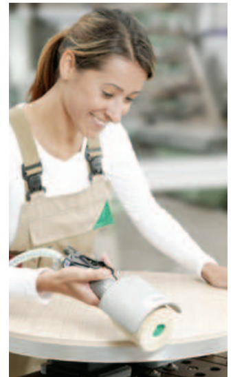
Air pressure-operated polishing of the radius and removal of material residues.
